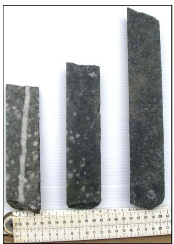
**Figure 7-5: Host rock and alteration associated with molybdenum mineralization** Left to right: quartz-feldspar porphyry host rock; mafic volcanics with epidote-sericite alteration and quartzphenocrysts; granitoid with epidote-sericite alteration.
