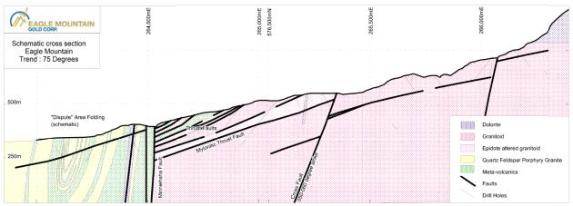
Figure 7-6: Schematic section looking north-northwest illustrating thrust bound lithological domains (EMGC, 2012)
