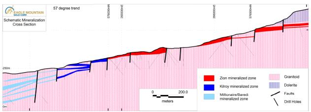
Figure 7-11: Northeast (057) trending section looking northwest illustrating gold mineralization zones (EMGC, 2012)
