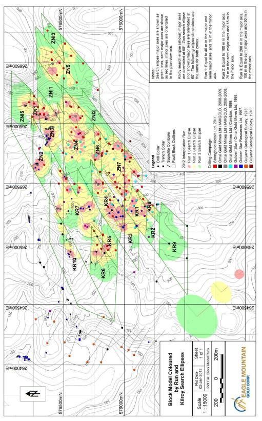
Figure 14-11: Block model coloured by run and Kilroy search ellipses.
