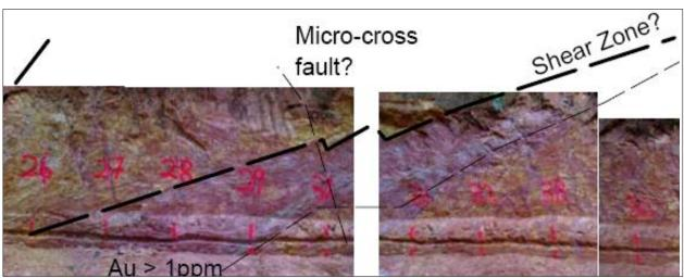
Red numbers refer to 1m samples Figure 7-8: Example of a small zone of low angle shear controlled mineralization
