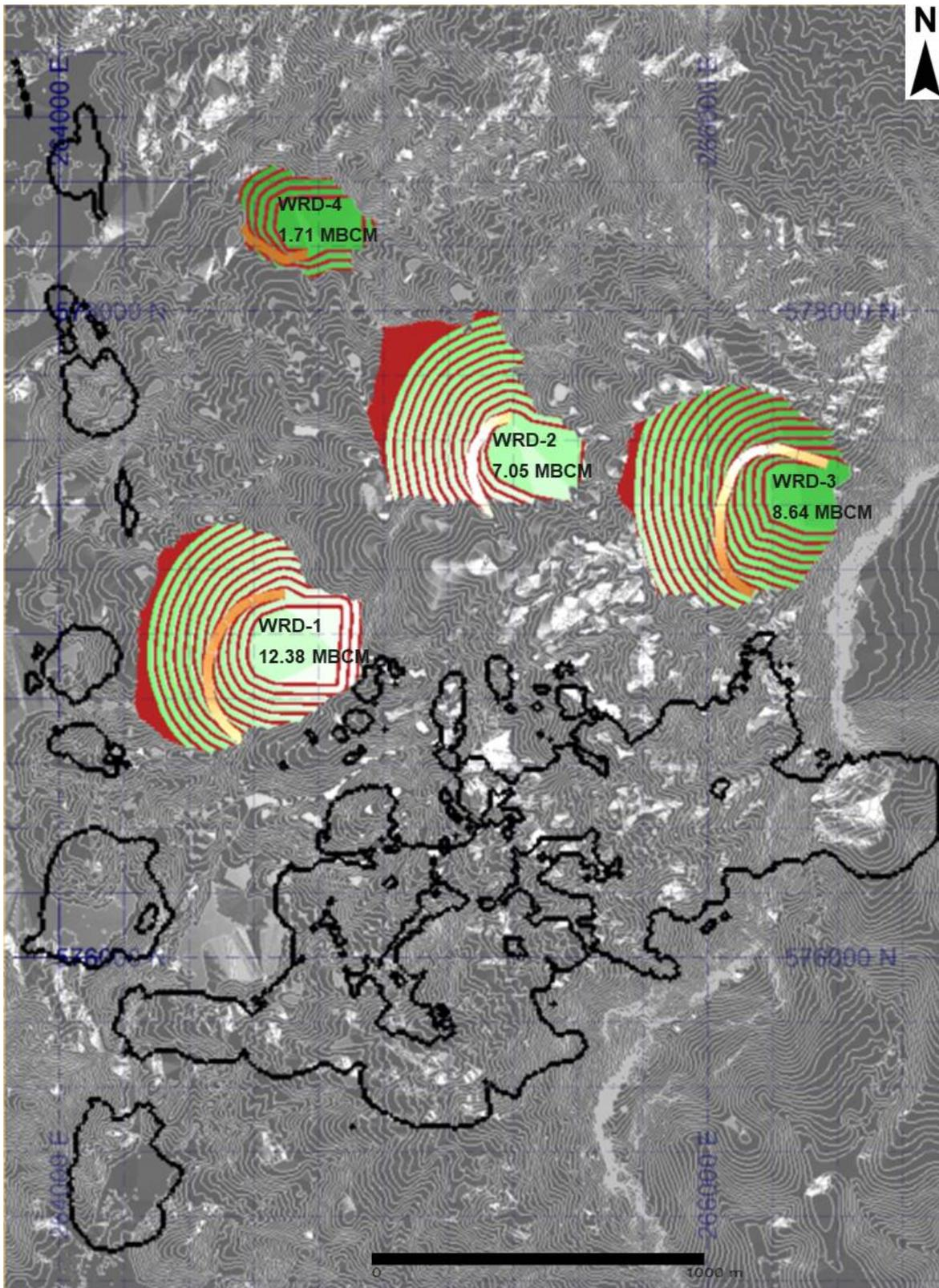
The total volume of waste rock produced in the open pit mining operations is based on the selected optimized pit shells created for the PEA, which will be equivalent to approximately 28 Mm<sup>3</sup>.
