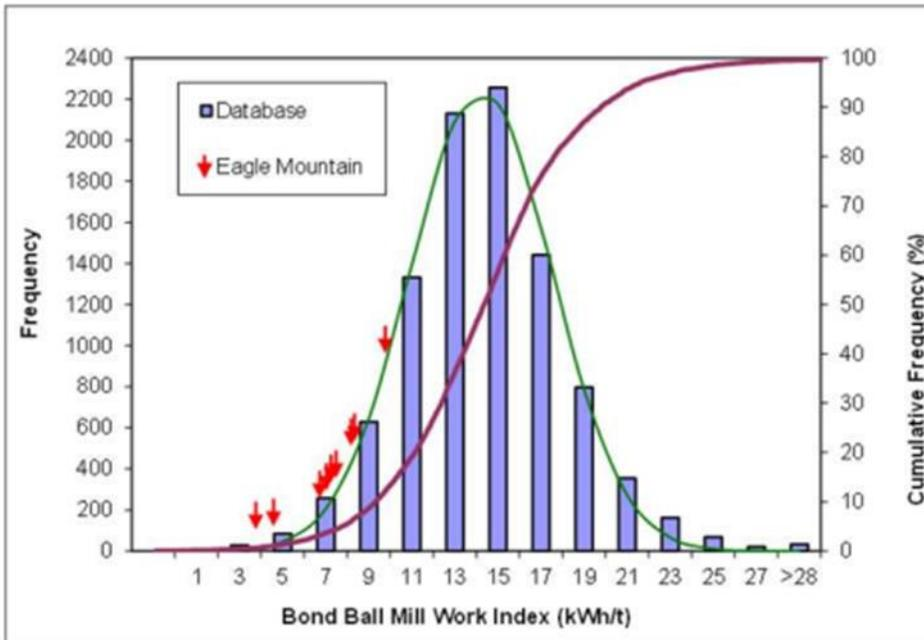
The overall BWI values of the saprolite samples ranged from 3.7 kWh/t to 9.7 kWh/t, which classifies them as very soft when compared to the SGS database. Samples No. 15 and No. 16 (Salbora saprolite) were among the softest samples in the SGS database. The results for the saprolite rock show that the overall grinding energy requirements to be very low.
