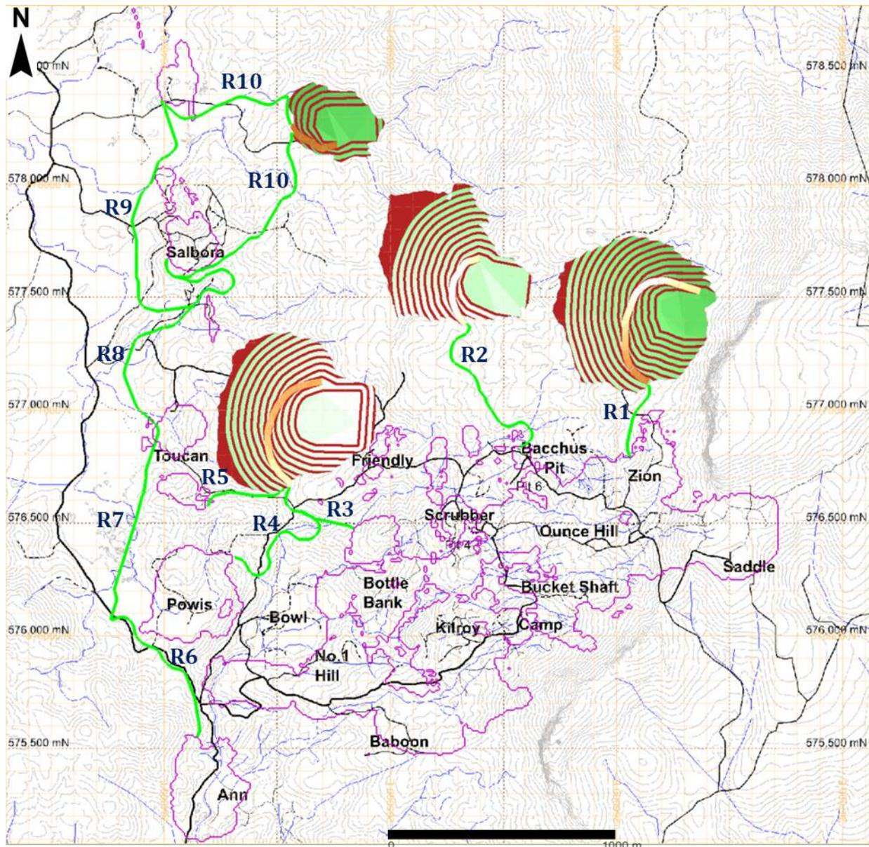
At an estimated cost of approximately US\$250/metre, the construction of the primary haulage roads/ramp system of approximately 14 km (about 8.7 mi) would require approximately US\$3.5 millions of road construction during pre-production.
