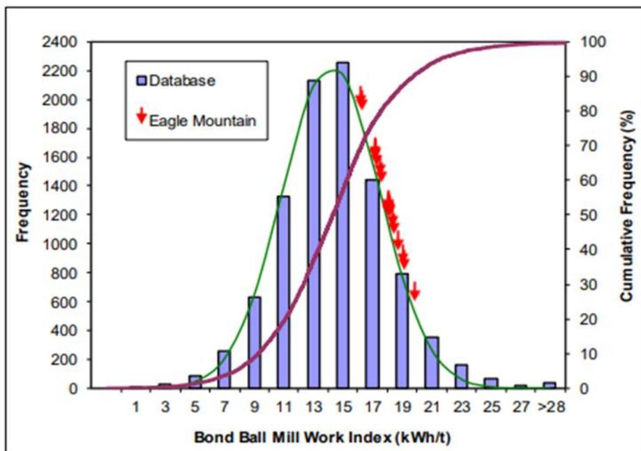
With BWI values ranging from 16.2 kWh/t to 19.9 kWh/t, the fresh rock samples fell in the moderately hard to hard range compared to the SGS database. With a standard deviation of 0.7, this indicates a homogeneous hardness across the deposit samples tested.
