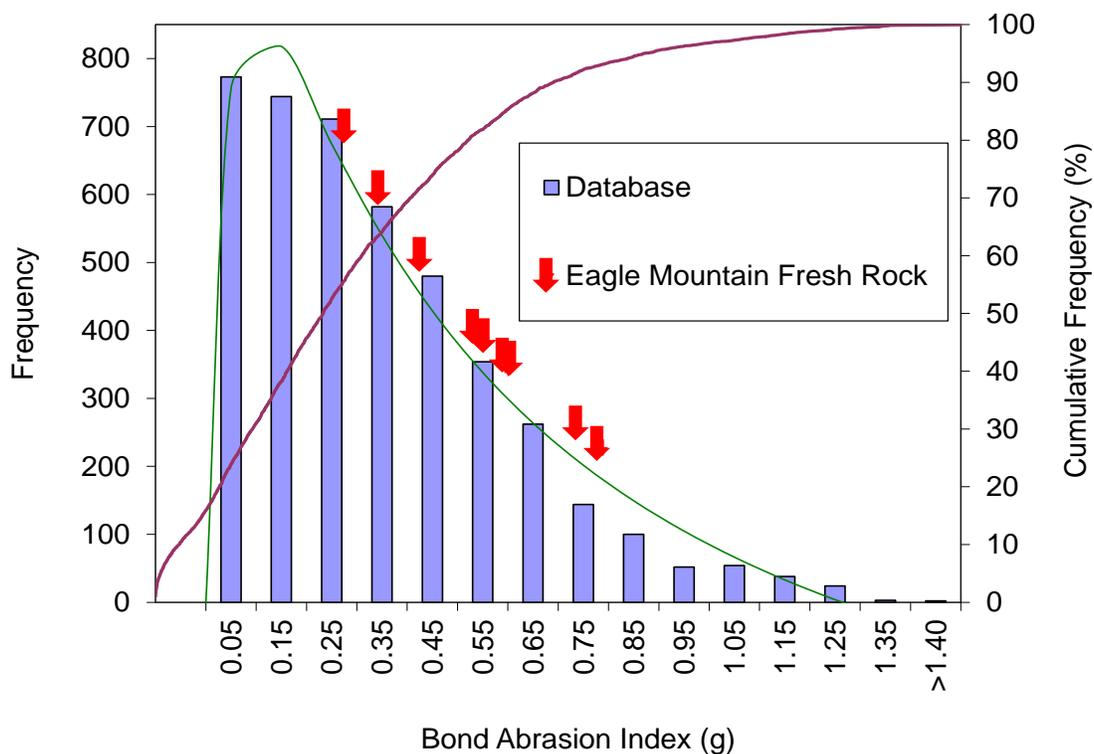
The results of the abrasion test performed are very scattered. This indicates that each area is quite different in terms of the abrasion.
