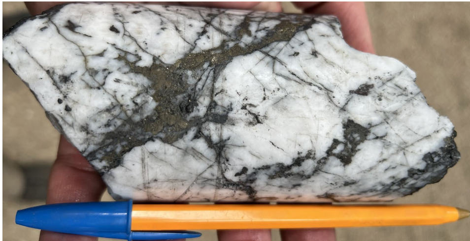
Figure 7-8 SVS Mineralization Overprinted on QS Vein, Mina Francisco, Drillhole LC22-549, Assayed 8.7 g Au/t and 49.2 g Ag/t
