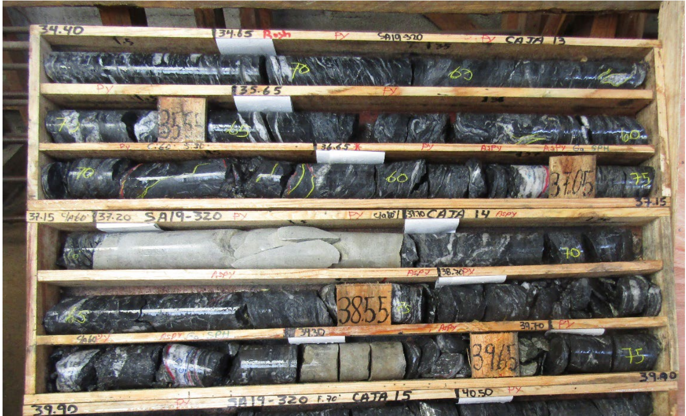
A typical dike interval is shown by the light coloration from 37.2m to 37.7m and 39.3m to 39.5m.
