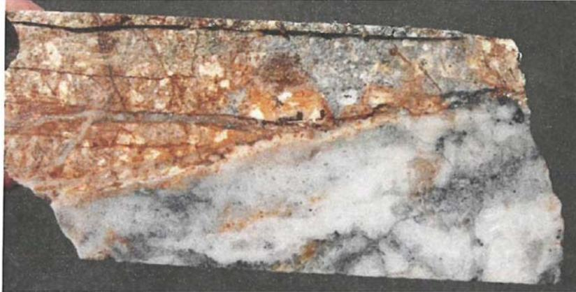
**Figure 7.10: An Example Quartz Vein Material with Bladed Texture from Calcite Replacement and Showing Limonite Staining (oxidation) along a Joint Plane (drillhole AR-69C, 80.77 m)**
